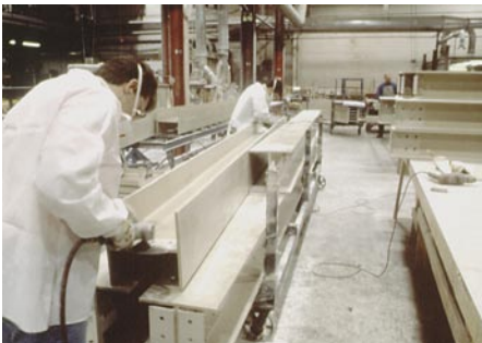
Beams are prepped before bonding connections together.
